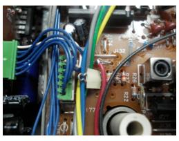
Route retrofit PCB wires as shown
