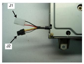
Connect J1 to the Kennedy Switch assembly you installed.
